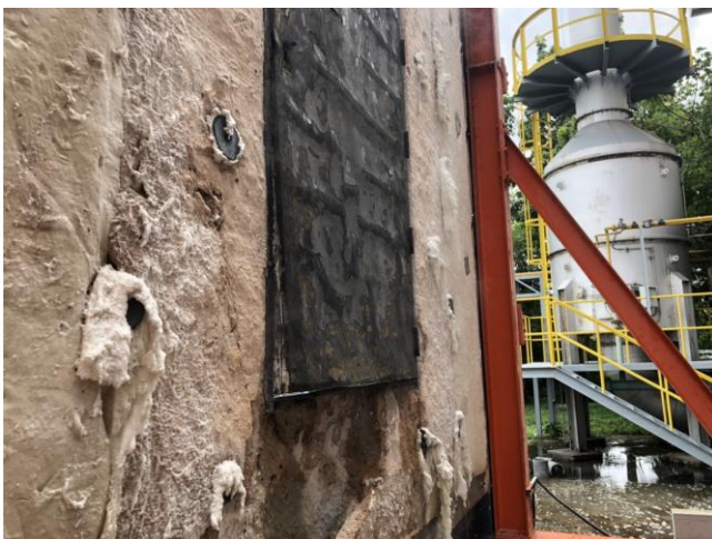
Figure E-4: The specimen after the hose stream test
