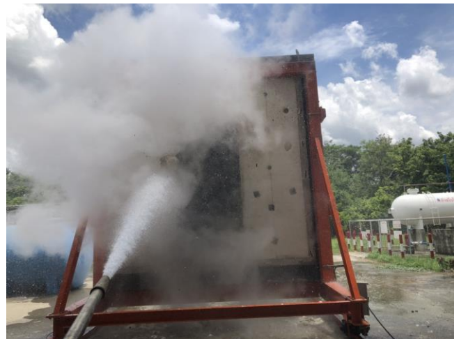
Figure E-3: The hose stream test
