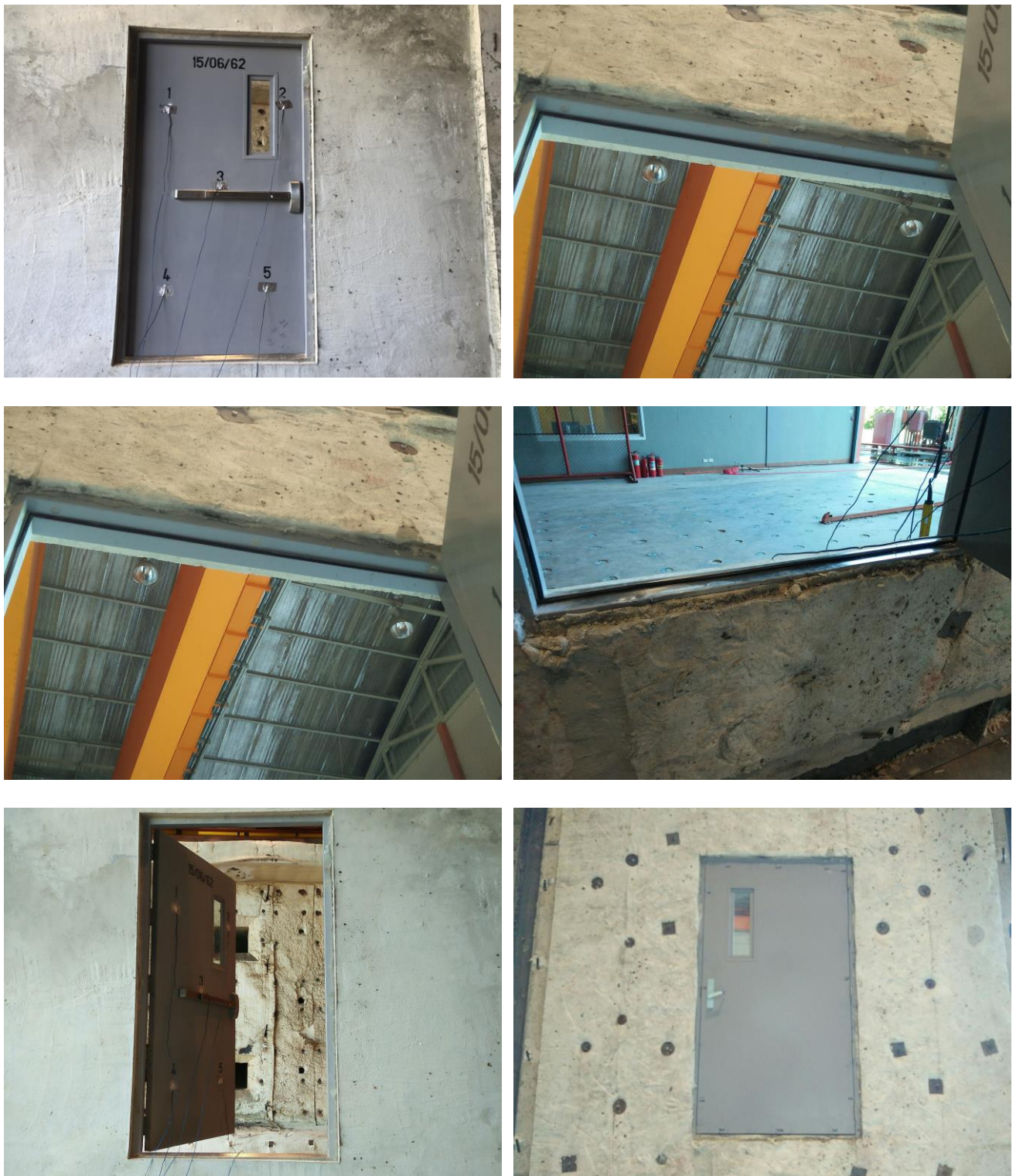
Figure E-1: Specimen preparation prior to the test
