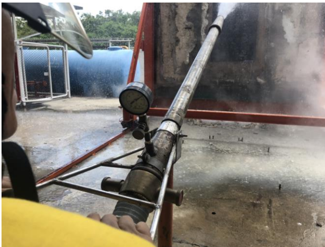
Figure E-3: The hose stream test
