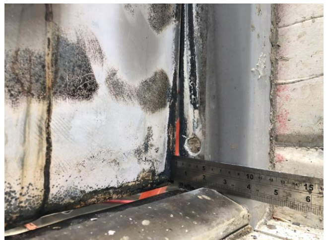
Figure E-4: The specimen after the hose stream test
